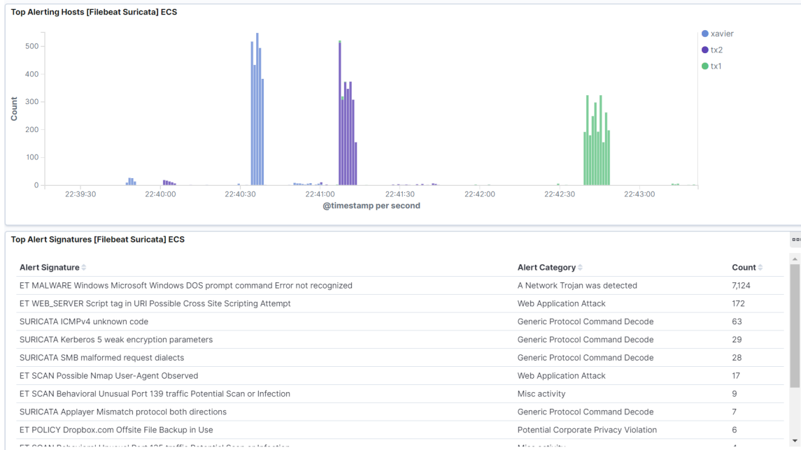
Figure 52: Kibana Dashboard with all alerts reporting. The timestamps are different due to slight wall clock drift between devices
